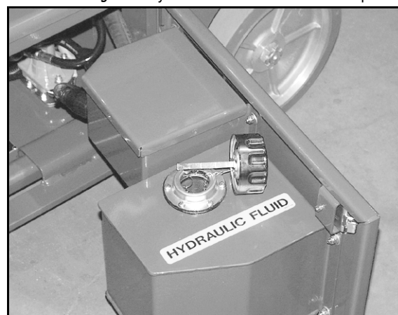
Figure 8: Hydraulic Fluid Reservoir and Dipstick
